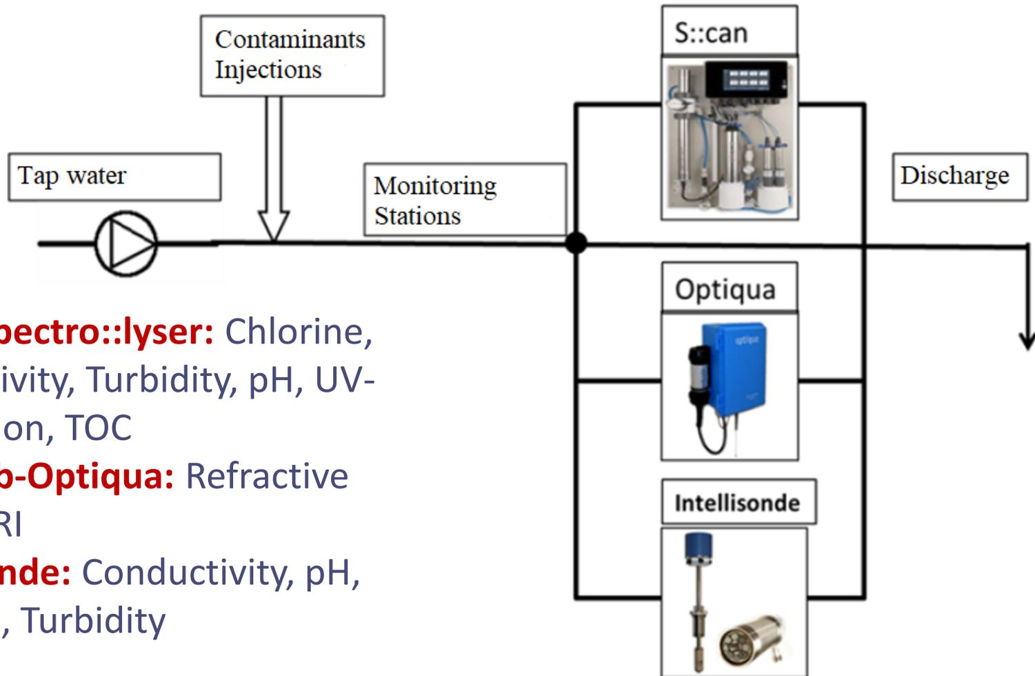
**S::can-spectro::lyser:** Chlorine, Conductivity, Turbidity, pH, UV-Absorption, TOC
