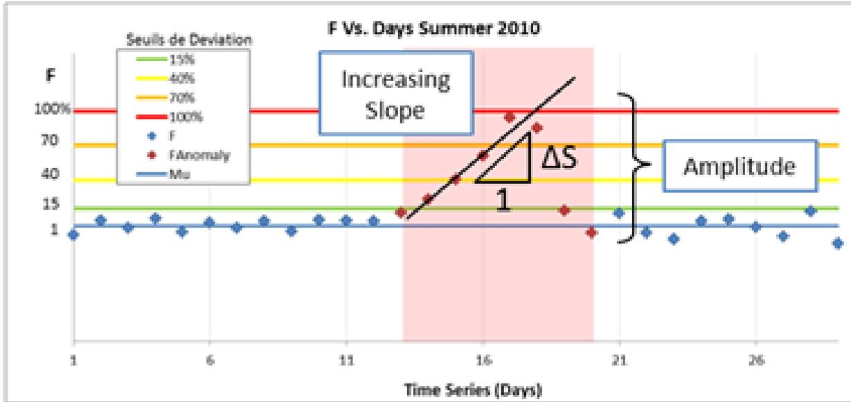
Normalization of MNF data to the average (F) & Deviations from the threshold in a Leak Likelihood Assessment
